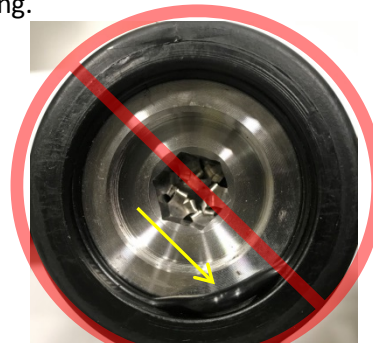
O-ring pinched and displaced
