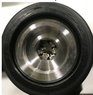
O-ring properly seated against punch
